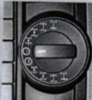
Relay switch for transfer case and differential locks.
